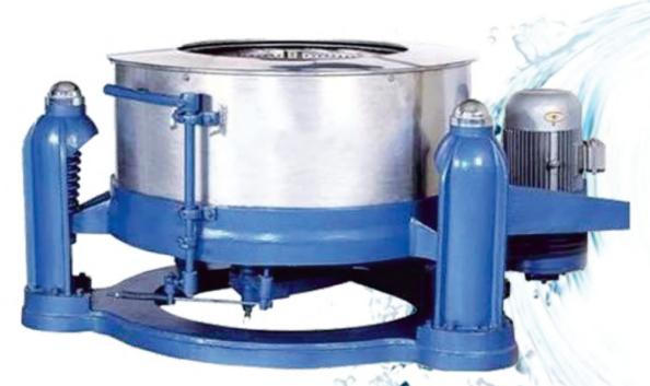
Inner rotating drum is of Stainless steel with close perforations for efficient water removal, the outer stationary basket is made of two halves, the upper part is of Stainless steel and the lower part is of heavy gauge Mild steel duly galvanized and painted for long life.
