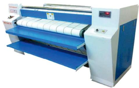
GEI FLAT WORK IRONERS are used to press bed sheets, pillow cases, table, linens, etc automatically. It's primary purpose is to remove wrinkles and they also dry the linens at the same time. The ironer is provided with a large heated roller, the linen are fed into the roller to iron and dry them. The feeding and heating belts are of Nomex brand.
