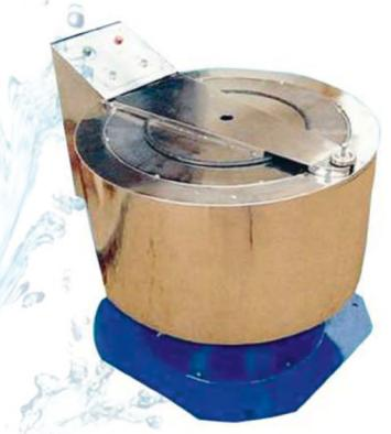
The outer drum is of stainless steel with electrical panel, and the door is interlocked for operator's safety. The machine has the feature of DC injection braking for efficient and trouble free performance.
